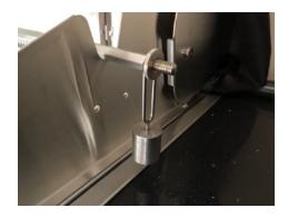
**6.** Screw the washer onto the rod end so that the balance weight can still spin freely on the rod.
