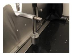
**5.** Install the balance weight onto the threaded end of the rod.
