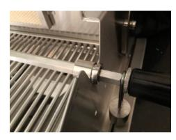
**11.** Align the slot on the slotted nut with the upper firebox support.
