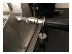
**8.** Install the slotted nut loosely onto the rod and slide down toward the handle.
