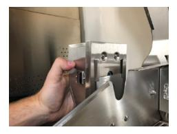
**3.** Place the motor into the mounting bracket with the on/off switch to the front by sliding down onto the bracket.
